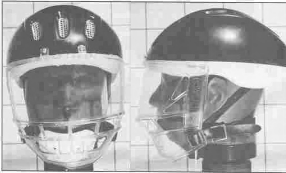
Figure 4. Micro-shell helmet with polycarbonate faceguard attached.
